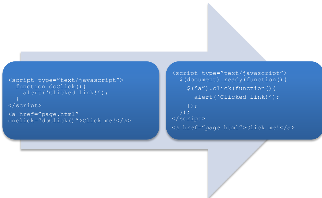
Figure 4 - Traditional Embedded JavaScript (left) and jQuery-based JavaScript (right) applied to a click event
